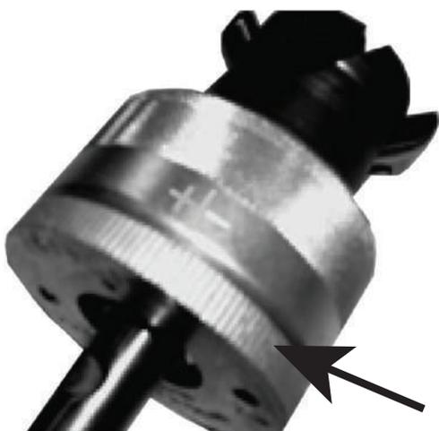
2. To enlarge the outlet rotate the conical cover with respect to the cover plate in plus (+) direction. Hold the cover plate stationary. To make a smaller outlet rotate the conical cover in minus (-) direction while holding the cover plate stationary. One notch on the cover-plate equals to 0.01" or 0,25 mm on the forming pin span.
