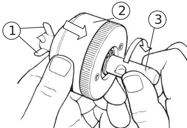
To extend the forming pins (1) press the cover (2) in direction of the shank. Twist the shank (3) at the same time clockwise until a positive stop is reached, and the forming pins extend.
