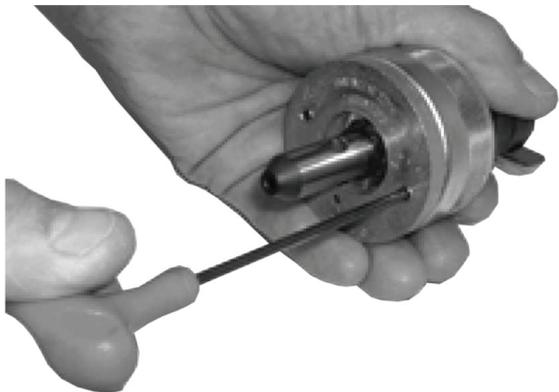
1. Loosen the screws on the cover plate by about one circle using a 3 mm hexagon wrench that is supplied with the T-DRILL package.
