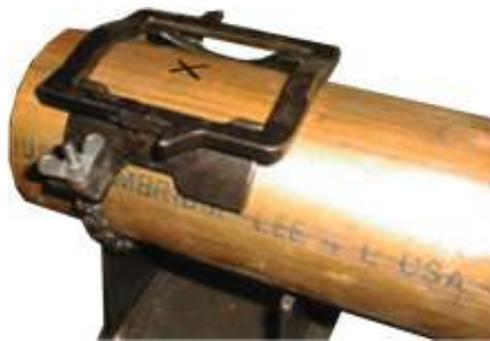
2. Attach counterplate to the tube where annealing has been done.
