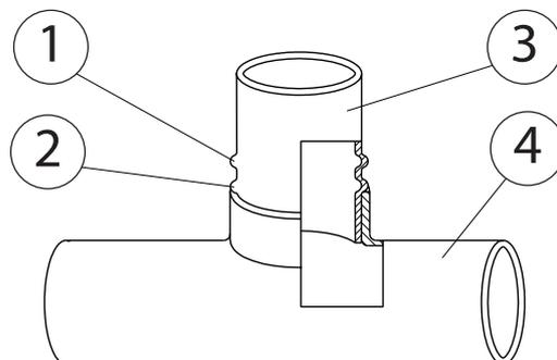
1. Point of inspection, 2. Depth stop, 3. Branch tube, 4. Run tube
