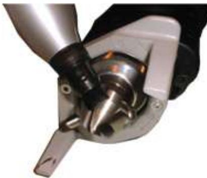
3. Lubricate forming pins and cutting edges on T-DRILL head.
