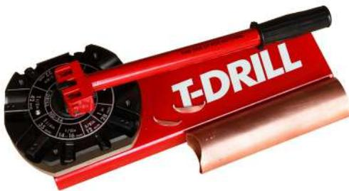
6. Notch and dimple both sides of branch tube.
