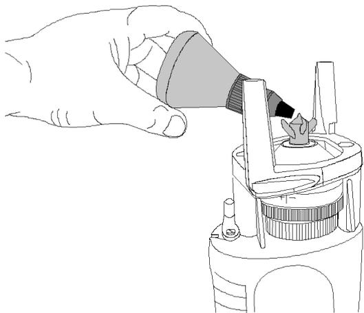
4. Lubricate the T-DRILL head before every tee forming operation! Extend the forming pins and lubricate them as well as the cutting edges of the T-DRILL head as illustrated. Always use T-DRILL lubricant.
