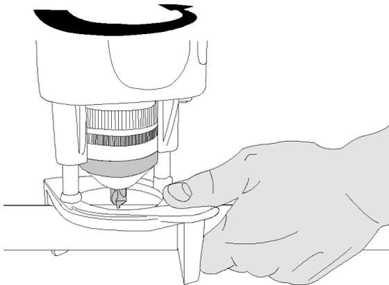
7. Pull the support legs out and place the tube support firmly onto the point where the tee is to be formed on the tube, as shown on the illustration. Press the tube support with the thumb against the tube and twist the machine counterclockwise at the handle of the tool. This centers the T-DRILL head onto the tube.
