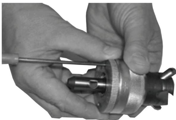
3. Tighten the two screws on the cover plate and check the adjustment either by measurement across the pins or by forming a trial outlet.
