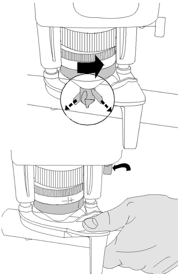
9. Extend the forming pins on the T-DRILL head by pressing the conical cover towards the tool and rotating it counterclockwise until the T-DRILL head locks into the tee forming position.
