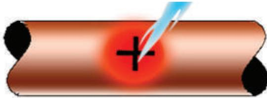
1. Anneal the area where outlet is to be formed to a dull red. The area will remain annealed even when cool. It is not necessary to form the outlet on hot tube!
