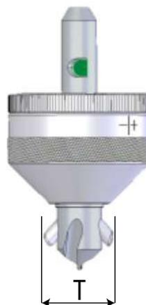
*Check the forming pin span diameter "T" with an adjusting ring or slide gauge.*
