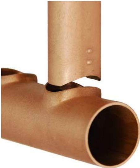
7. Align dimples with the run of the tube after insertion into the outlet. Braze the joint.
